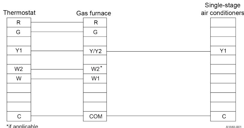
**Figure 21: Standard ECM furnace and premium multi-stage AC**
