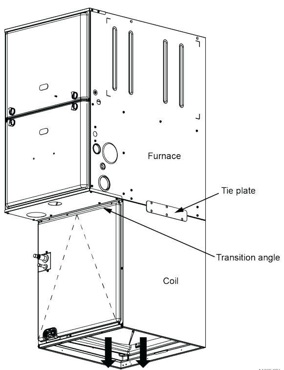
**Figure 7: Horizontal right application of the coil with the furnace**
