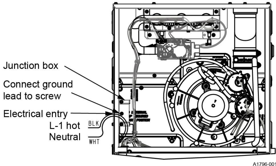
1. Provide a power supply separate from all other circuits. Install overcurrent protection and a disconnect switch in accordance with local and national electrical codes. Locate the switch close to the unit for convenience in servicing.
