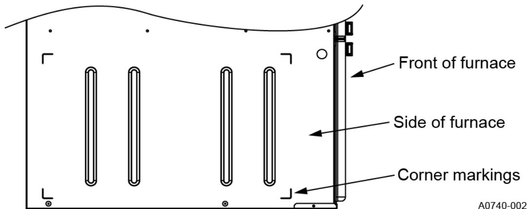
Install the side filter rack following the instructions provided with that accessory. If filters are provided at another location in the return air system, the ductwork can be directly attached to the furnace side panel.
