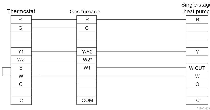
**Figure 19: Standard ECM furnace and multi-stage HP**
