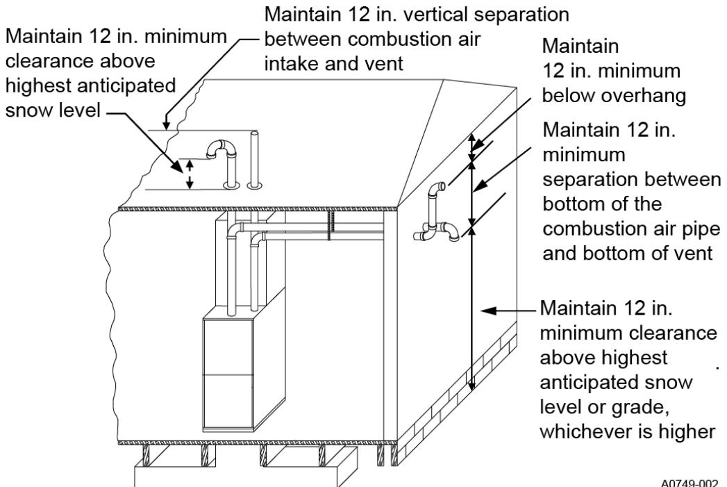
**Figure 31: Termination configuration - two pipe basement**
