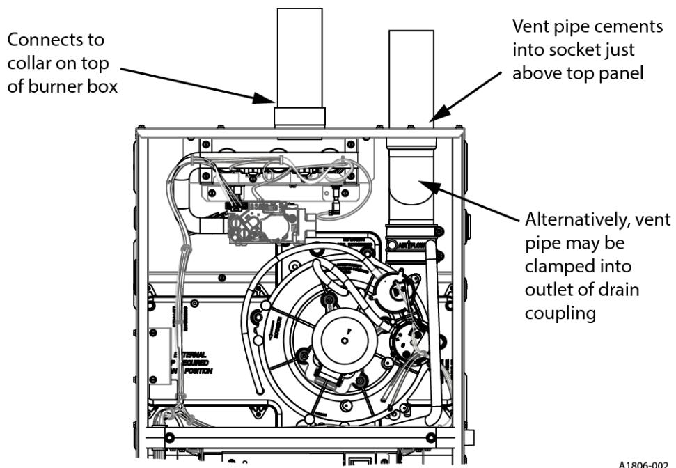
Locate the combustion air intake pipe either through the wall (horizontal or side vent) or through the roof (vertical vent). Do not locate side vented systems where trees or shrubs can block or restrict supply air from entering the terminal.
