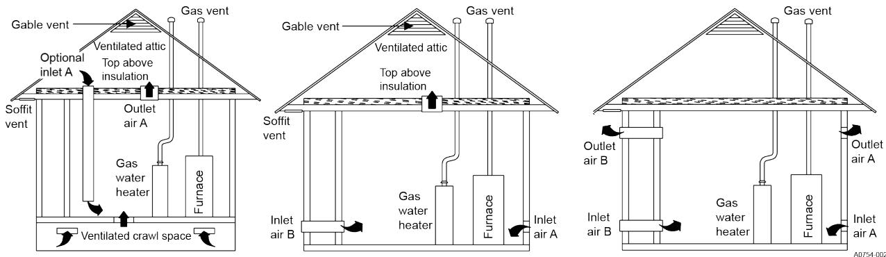
**Figure 37: Combustion airflow path through the furnace casing**
