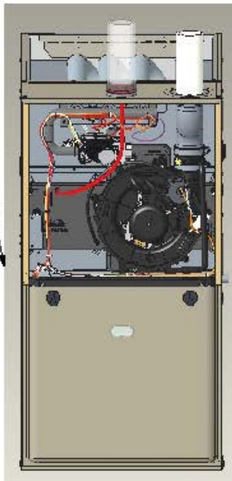
For 100k and 120k input furnaces, the condensate drain is plumbed toward the left casing outlet from the factory
